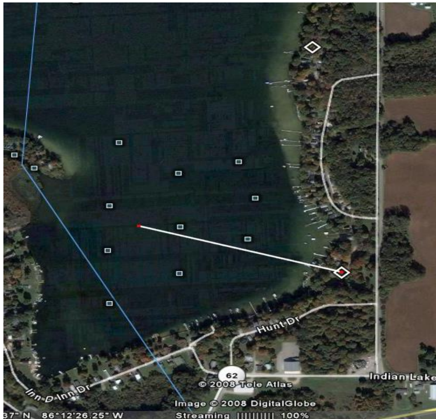
Figure 8. Laminar Flow system design for Indian Lake South Basin designed by Clean-Flo (2010).
